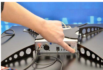
8. Push Volume Knob if green LED does not flash even when powered
