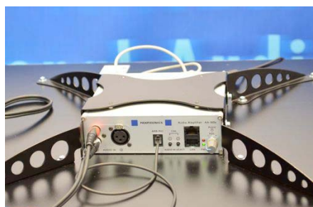
7. Connect ambient microphone to amplifier ( Green LED starts blinking when powered )
