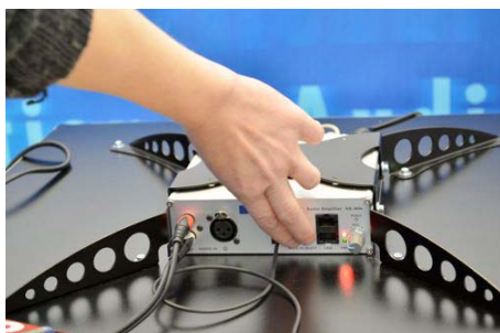
10. Press calibration buttons simulatniously to set ambient control
