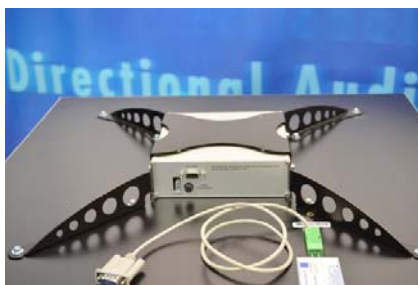
2. Connect D-connector to panel
