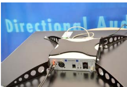
5. Connect RCA cable to amplifier
