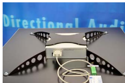
3. Connect D-connector to amplifier
